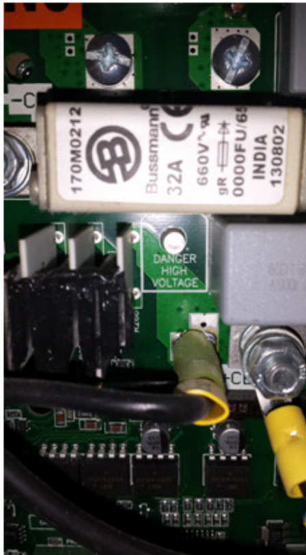
Picture 2 – DANGER LED off = safe to work on.
